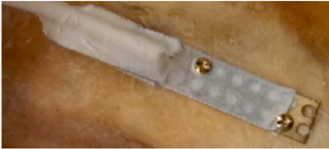
Fig. 12. Encapsulated sensor attached to the bone with screws placed like indicated at the numerical model. Here, part of the optical cable wrapped by silicone tube and the sensor covered by the tape microporous can be seen.
